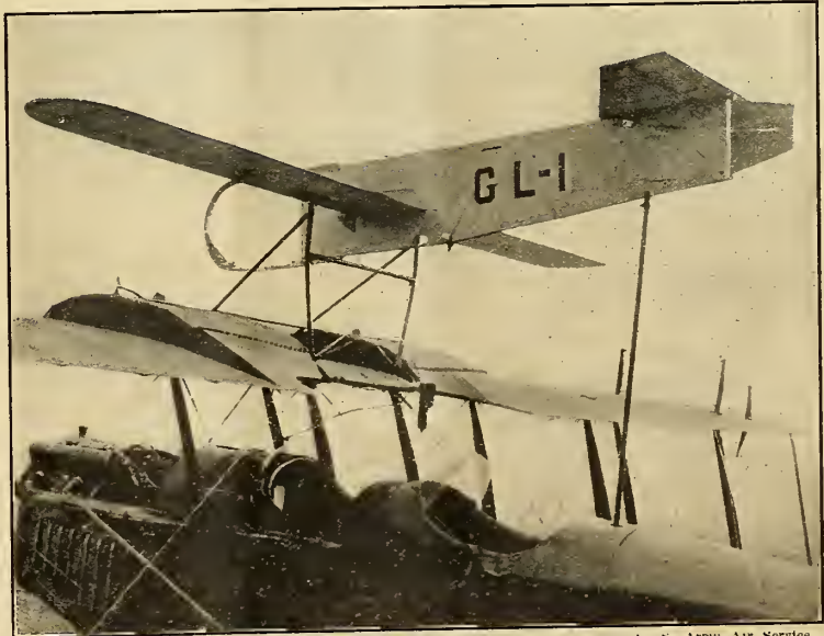
Target glider of the U. S. Army Air Service mounted on a "Jenny"
